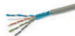
03061.E Cat. 5e F/UTP cable, shielded, 4-pair, 24 AWG, LSZH-sheath, CPR Eca class, suitable for I category cables (U0 = 400 V), grey - 305 m
