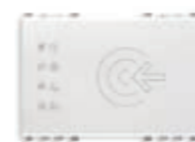
20457.B Transponder card reader for installation outside rooms, KNX standard, 2 NO 4 A 24 V~ relay outputs, 2 inputs, power supply 12-24 V~ 50/60 Hz and 12-24 Vdc (SELV), white - 3 modules. Supplied without transponder card. Depth: 37 mm
