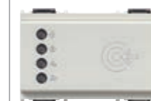
16927.B Transponder card reader for installation outside rooms, KNX standard, 2 NO 4 A 24 V~ relay outputs, 2 inputs, power supply 12-24 V~ 50/60 Hz and 12-24 Vdc (SELV), white - 3 modules. Supplied without transponder card. Depth: 36,5 mm
