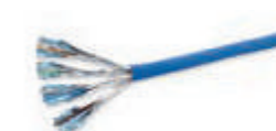
03086.B2 Cat. 6A F/FTP cable, shielded, 4-pair, 23 AWG, LSZH sheath, CPR B2ca class, blue - 500 m
