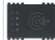
19457 Transponder card reader for installation outside rooms, KNX standard, 2 NO 4 A 24 V~ relay outputs, 2 inputs, power supply 12-24 V~ 50/60 Hz and 12-24 Vdc (SELV), grey - 3 modules. Supplied without transponder card. Depth: 37 mm
