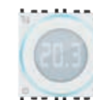
02971.B Dial thermostat (heating and air conditioning), 2- and 4-pipe system management, 3-speed and proportional fan coil control, class I (contribution 1%) in ON/OFF mode, class IV (contribution 2%) in PID mode, can be interfaced with actuator 01466.1 to make a class V modulating room thermostat (contribution 3%), 1 input for sensor 20432, 19432, 14432 or 02965.1, white LED backlighting, white - 2 modules. Depth: 28,5 mm
