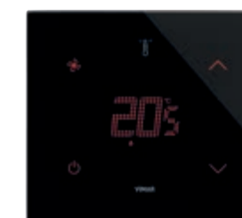
21514.F.76 Touch screen thermostat (heating and air conditioning), 3-speed and proportional FAN COIL control, class I (contribution 1%) in ON/OFF mode, class IV (contribution 2%) in PID mode, can be interfaced with actuator 01466.1 to make a class V modulating room thermostat (contribution 3%), 1 input for sensor 20432, 19432 or 14432 or wired sensor 02965.1, 1 programmable digital input, RGB LED backlighting, black diamond - 2 modules. Depth: 30,2 mm
