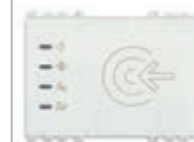
19457.B Transponder card reader for installation outside rooms, KNX standard, 2 NO 4 A 24 V~ relay outputs, 2 inputs, power supply 12-24 V~ 50/60 Hz and 12-24 Vdc (SELV), white - 3 modules. Supplied without transponder card. Depth: 37 mm
