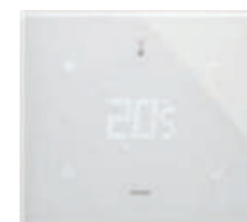
21514.F.70 Touch screen thermostat (heating and air conditioning), 3-speed and proportional FAN COIL control, class I (contribution 1%) in ON/OFF mode, class IV (contribution 2%) in PID mode, can be interfaced with actuator 01466.1 to make a class V modulating room thermostat (contribution 3%), 1 input for sensor 20432, 19432 or 14432 or wired sensor 02965.1, 1 programmable digital input, RGB LED backlighting, white diamond - 2 modules. Depth: 30,2 mm
