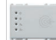
14457.SL Transponder card reader for installation outside rooms, KNX standard, 2 NO 4 A 24 V~ relay outputs, 2 inputs, power supply 12-24 V~ 50/60 Hz and 12-24 Vdc (SELV), Silver - 3 modules. Supplied without transponder card. Depth: 36 mm
