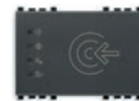
20457 Transponder card reader for installation outside rooms, KNX standard, 2 NO 4 A 24 V~ relay outputs, 2 inputs, power supply 12-24 V~ 50/60 Hz and 12-24 Vdc (SELV), grey - 3 modules. Supplied without transponder card. Depth: 37 mm
