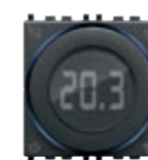
02971 Dial thermostat (heating and air conditioning), 2- and 4-pipe system management, 3-speed and proportional fan coil control, class I (contribution 1%) in ON/OFF mode, class IV (contribution 2%) in PID mode, can be interfaced with actuator 01466.1 to make a class V modulating room thermostat (contribution 3%), 1 input for sensor 20432, 19432, 14432 or 02965.1, white LED backlighting, grey - 2 modules. Depth: 28,5 mm
