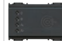
16927 Transponder card reader for installation outside rooms, KNX standard, 2 NO 4 A 24 V~ relay outputs, 2 inputs, power supply 12-24 V~ 50/60 Hz and 12-24 Vdc (SELV), grey - 3 modules. Supplied without transponder card. Depth: 36,5 mm
