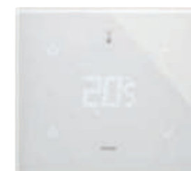
21514.S.70 Touch screen thermostat (heating and air conditioning), configurable STAR control, class I (contribution 1%) in ON/OFF mode, class IV (contribution 2%) in PID mode, can be interfaced with actuator 01466.1 to make a class V modulating room thermostat (contribution 3%), 1 input for sensor 20432, 19432 or 14432 or wired sensor 02965.1, 1 pro- grammable digital input, RGB LED backlighting, white diamond - 2 modules. Depth: 30,2 mm
