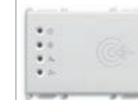
14457 Transponder card reader for installation outside rooms, KNX standard, 2 NO 4 A 24 V~ relay outputs, 2 inputs, power supply 12-24 V~ 50/60 Hz and 12-24 Vdc (SELV), white - 3 modules. Supplied without transponder card. Depth: 36 mm
