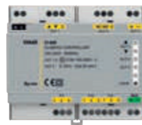
01465 Climate control device for heating systems, power supply 120-230 V~ 50/60 Hz, 3 inputs for PT100, PT1000 and NTC probes, 1 mixer valve control output, 1 0-10 V or (I) 4-20 mA output, 1 16 A 230 V~ change-over relay output, 6 x 17,5 mm modules
