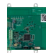
▲03832 Transceiver board, BUS connection to the control unit, 2 antennas for horizontal and vertical polarisation with antenna-diversity
