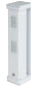
01740 Curtain-effect detector to protect entrances and openings such as doors, windows, covered terraces, corridors and French doors, short-range curtain-effect detection with adjustable lens up to 2 m or 5 m, PET immune, anti-masking function, 1 NO or NC 28 Vdc 0.1A relay output, surface mounting, 9.5-18 Vdc 20 mA power supply
