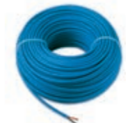
01840.E.B By-me system Bus cable for sound system, 2x0,50 mm 2 , with LSZH sheath, CPR Eca class, suitable for I category cables (U0 = 400 V), blue - 100 m
