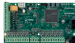
▲03800 By-alarm Plus control unit expandable to 25 zones
