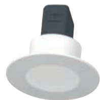
02692 UWB radar sensor, IoT technology on Bluetooth® wireless technology 5.0 standard for the creation of View Wireless mesh system, 1 solid state output for extra low voltage controls (SELV and non SELV), 1 input for external push button for output activation or to recall a scenario, 100-240 V 50/60 Hz power supply, installation in false ceiling
