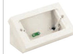
▲30784.B Tilted table mounting box, with variable height, for the installation of 4 modules. In the lowered version, connector blocks with a maximum depth of 32 mm can be installed; if you turn the cover the maximum depth extends to 44 mm. The socket outlet with USB, 30210. USB, cannot be installed. To be completed with mounting frame and cover plate.
